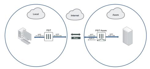
As per the above diagram the topology is consisted of a local FortiGate in a local environment with port5 configured as WAN and port 4 as LAN and a FortiGate located in Azure with port1 connected to WAN and port 2 connected to LAN.
